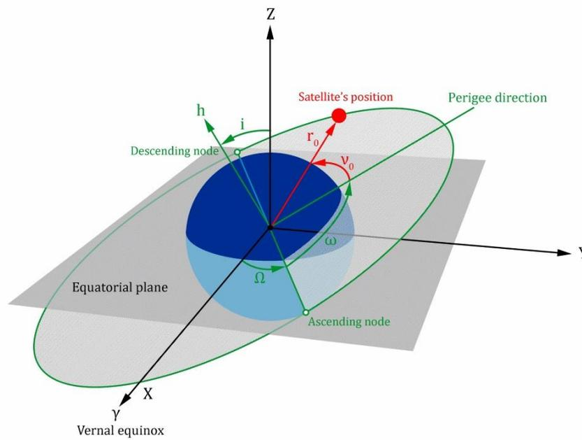
**Figure 25: Orbital analysis of the satellite**
